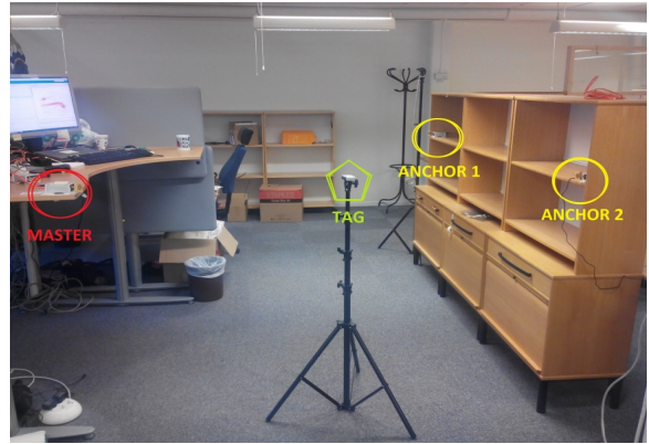
Fig. 6 Setup of OpenRTLS based prototype
