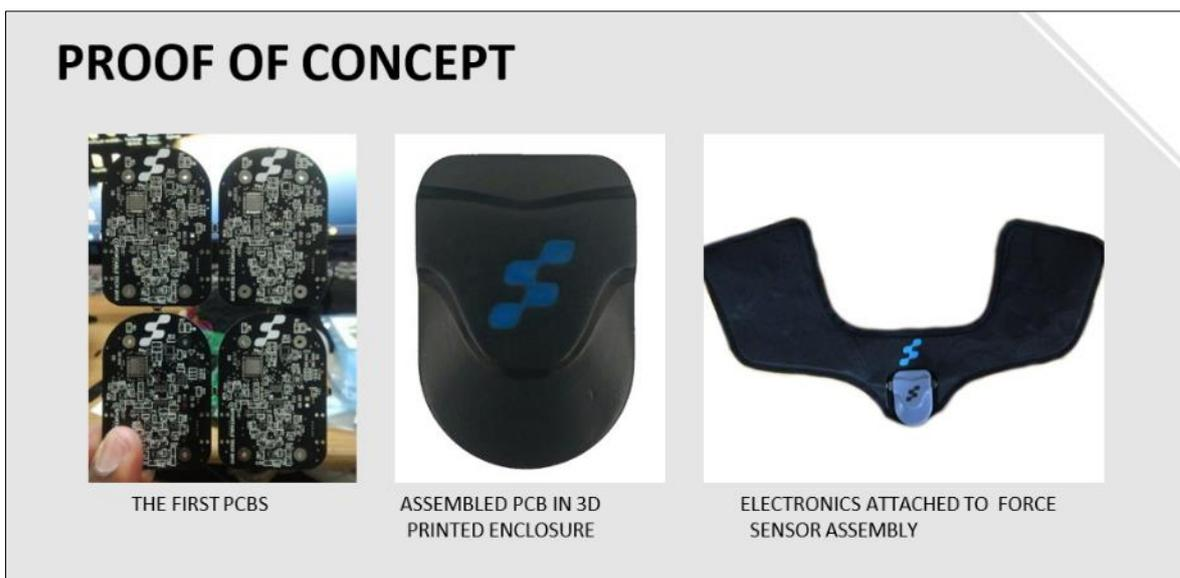
We sourced cables, connectors and components. We got our first custom circuit boards made and assembled. Another friend 3D printed us some enclosures which
