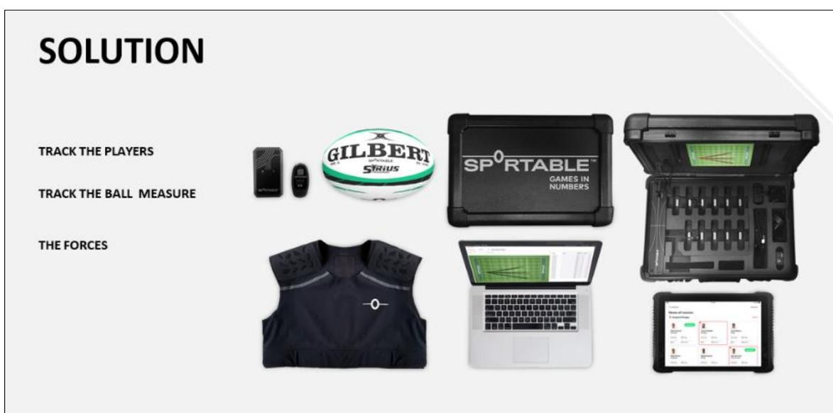
We get a lot of data from our hardware, and it is all streamed in real-time to a pitch-side server which converts the data, into useful information. For example, twenty times every second we get the ball's 3D position, velocity, acceleration, spin, we get its orientation as a quaternion, we get its compass reading, the barometric pressure and temperature. Similarly, for every player on the field we get the same data by we also get force and real-time heart-rate.
