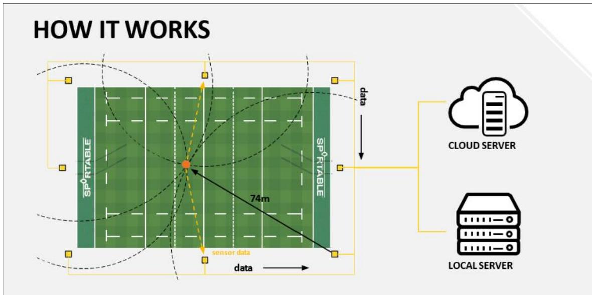
The network records either the time it took for those messages to travel from the anchors to the player and ball devices and back (which is called time of flight or ToF), or it records the time difference between a reference anchor receiving the messages and the rest of the anchors receiving the messages (which is called Time Difference of Arrival or TDoA).
